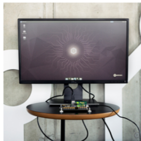
Linux GUIs on Zynq with FastVDMA, HDMI and Snickerdoodle
